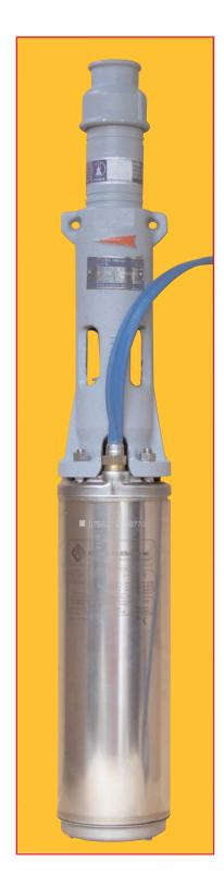
Progressive cavity (helical rotor) pumps designed for 4" borehole applications, handling clean or dirty water with entrained solids up to a max. 5mm diameter. Suitable for deep well applications from depths of 8m and more, they handle pumped media temperatures up to 30°C (larger motor/higher temperature models available) with acidity ranging from 6.5 to 12 pH.
