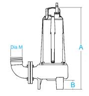
A range of heavy duty pumps designed for dirty water and sewage applications, combining excellent solids handling characteristics with long service life. All models are available in 400/3/50 with an additional 230/1/50 version of the 754 model. The 754 model features a low r.p.m. 4-pole motor which is particularly suited to abrasive media applications. Motor cylinder, tie rods, handle, bolts and motor shaft: Stainless steel
